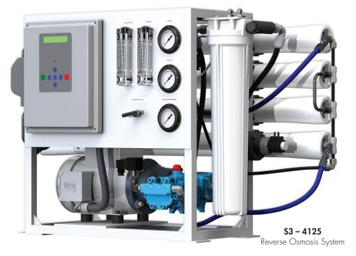
The S3 – Series is also equipped with premium components, which include a 316L SS plunger–type pump for high performance, a high grade corrosion resistant aluminum frame, a programmable computer controller with many built–in features and fiberglass membrane housings for durability.
